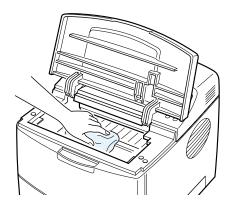
**CAUTION:** To prevent damage to the toner cartridge, do not expose it to light for more than a few minute. Cover it with a piece of paper, if necessary. Also, do not touch the black transfer roller inside the printer.
